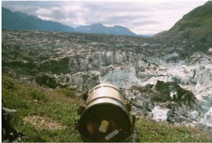
Figure 4.2 Photograph showing the barrel that holds the time lapse camera pointed directly at the ice dam. Note the copious amount of ice debris that collects in the basin after the flood.
